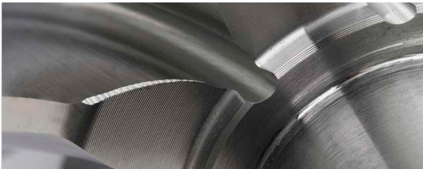
Fig. 8: Contour generated with many different positions of the deburring tool
