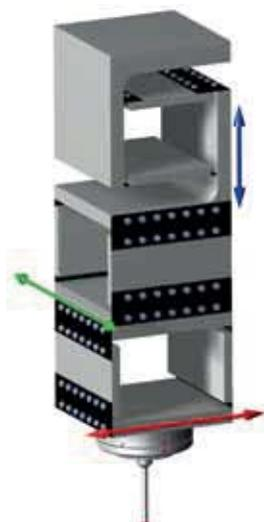
Fig. 4: Diagram of a conventional 3-D measurement system with serial kinematics
