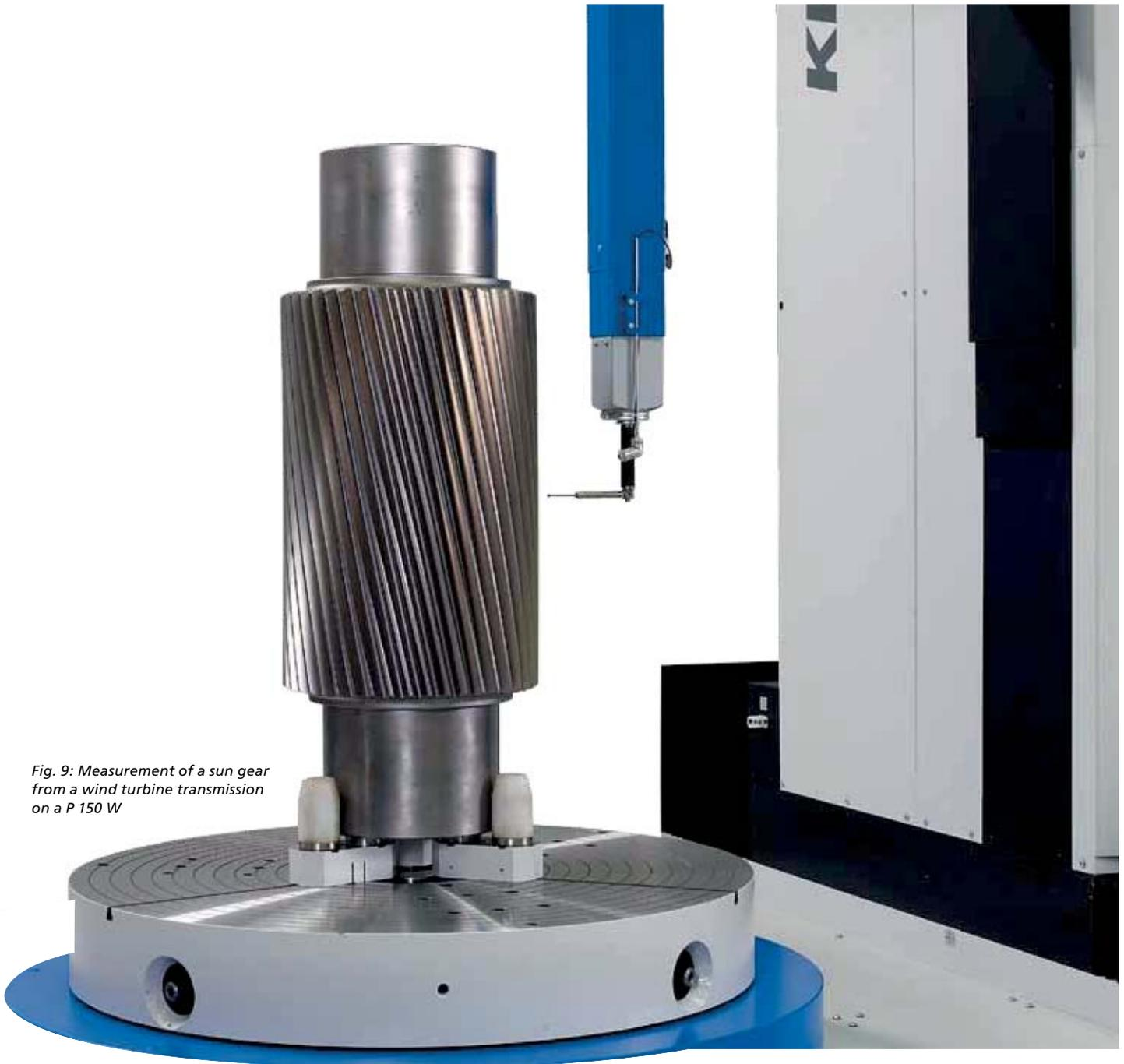
*Fig. 9: Measurement of a sun gear from a wind turbine transmission on a P 150 W*
