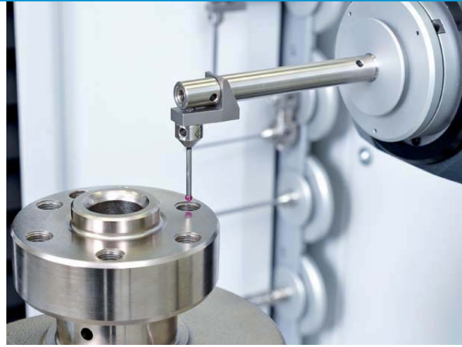
Fig. 2b: Drive flange testing (measurement of bore hole and angular position); the automatic probe change rack can be seen in the background.
