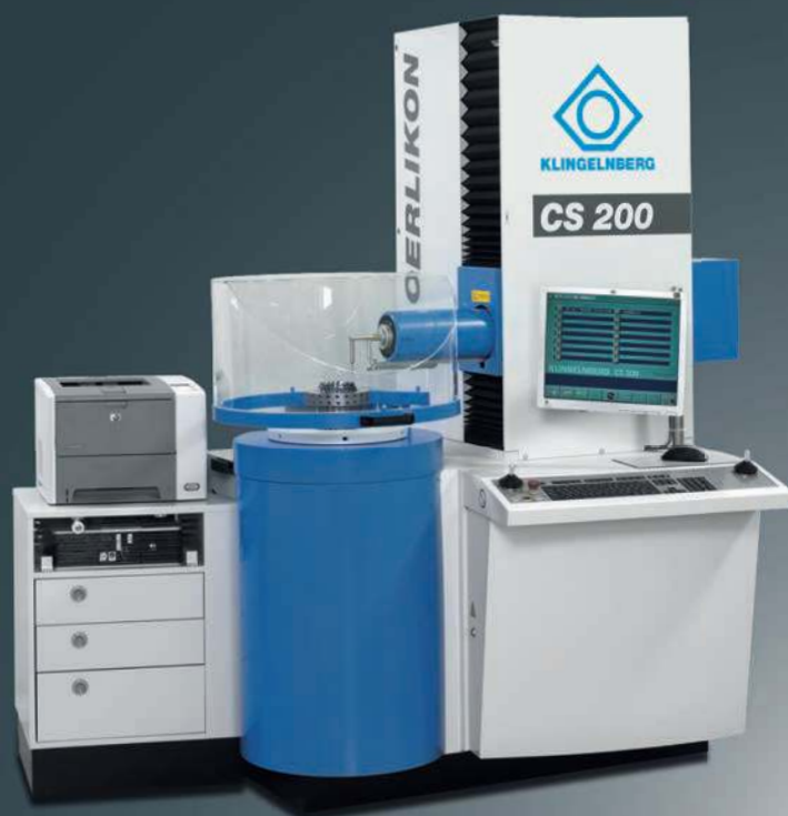
Oerlikon (奥利康) 刀盘安装和检查仪CS 200
