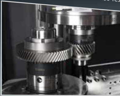
Gear Noise Check by Single-Flank, Torsional Acceleration & Structure Borne Noise Test
