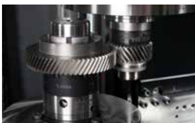
Gear noise testing by single flank, torsional acceleration and structure-borne noise testing.
