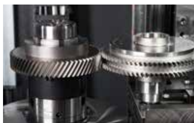
Testing of hardness distortions by the Helix test.
